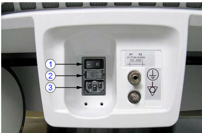
Figure 3-14 Circuit Breaker at rear of system
