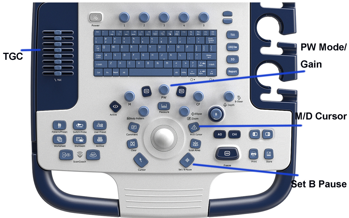
Figure 4-12 Controls available in Doppler Mode
