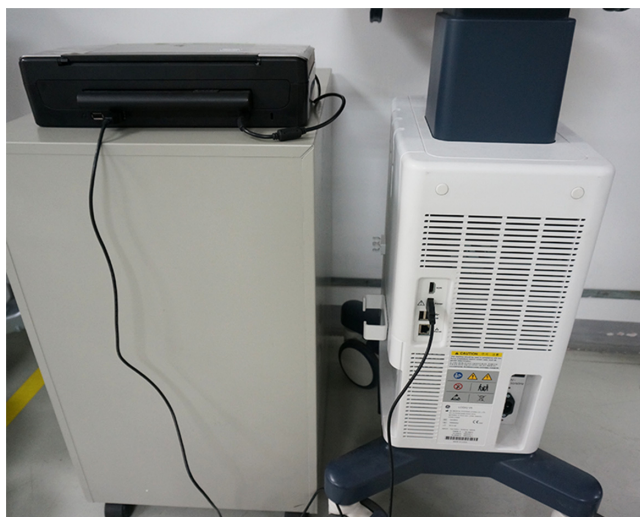
Figure 3-10 HP Officejet 100 printer to the system
