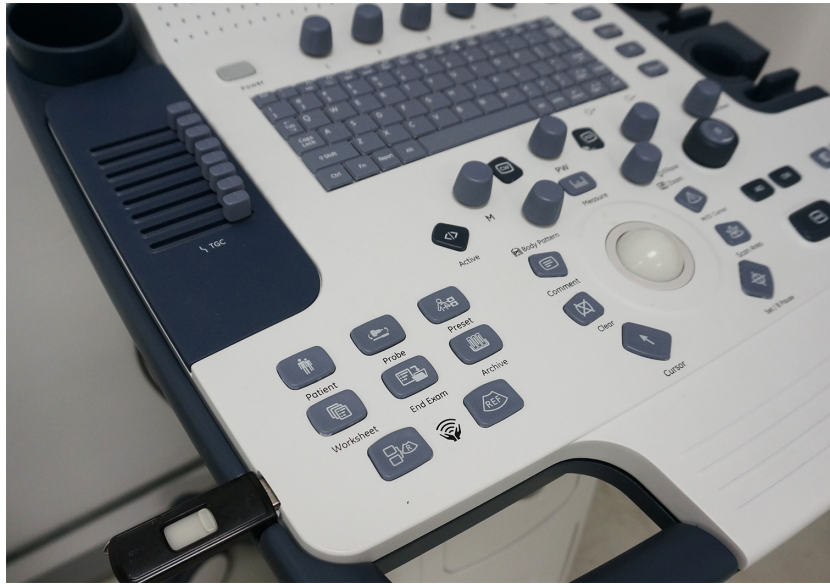
Figure 3-12 USB Memory Connection
