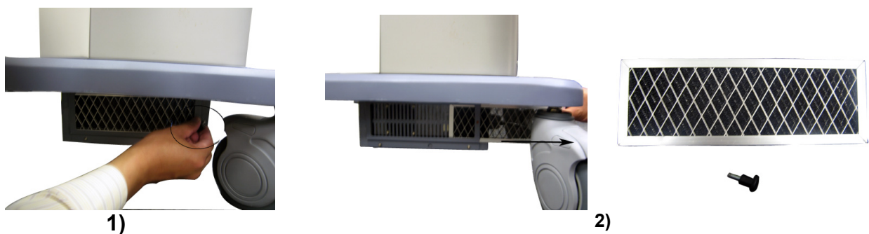
Figure 8-1 Air filter and Knob Screw Disassembly
