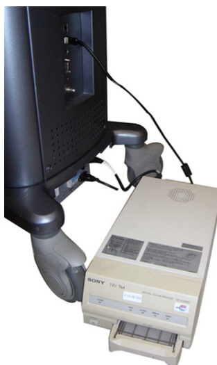
Figure 3-10 Connect color printer to the system
