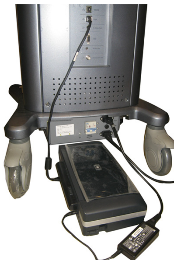
Figure 3-15 HP 470b Officejet printer Connection
