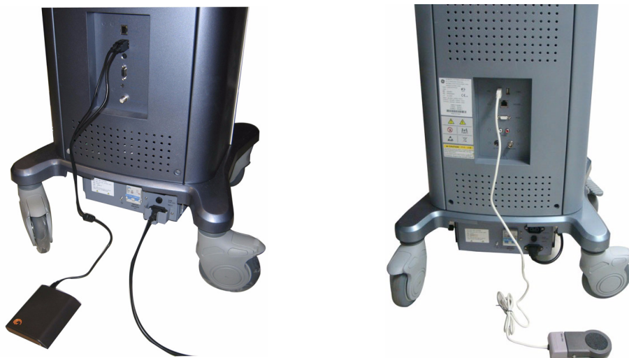
Figure 3-14 USB Hard Disk Connection
