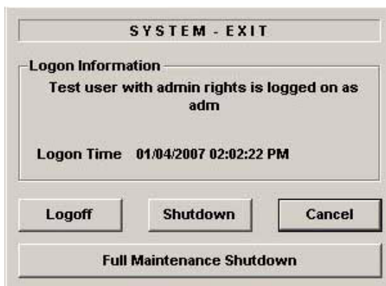
Figure 4-44 System Exit Window
