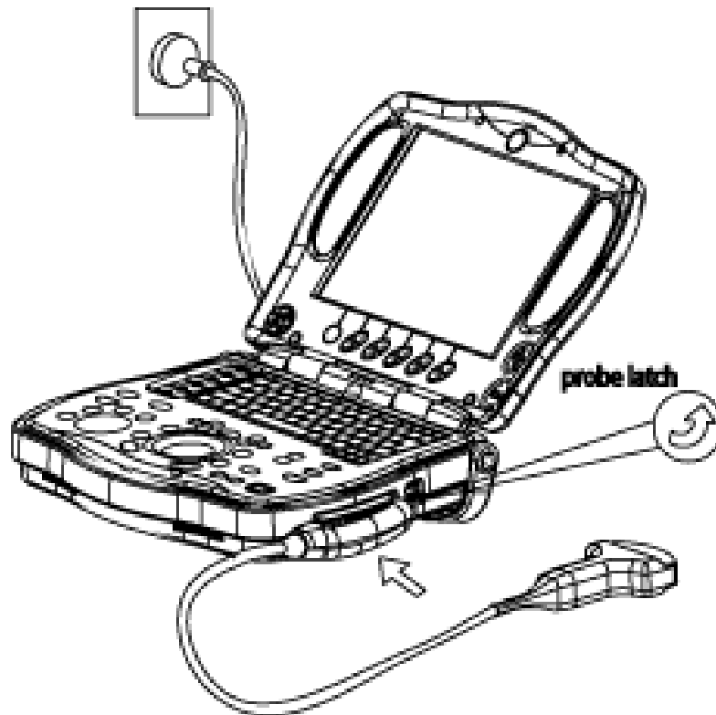
Figure 3-10 Connect the probe
