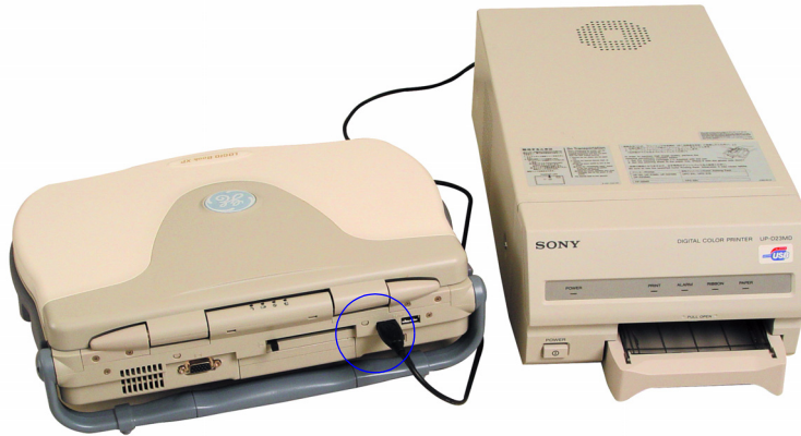
Figure 3-14 Connect digital color printer to the system
