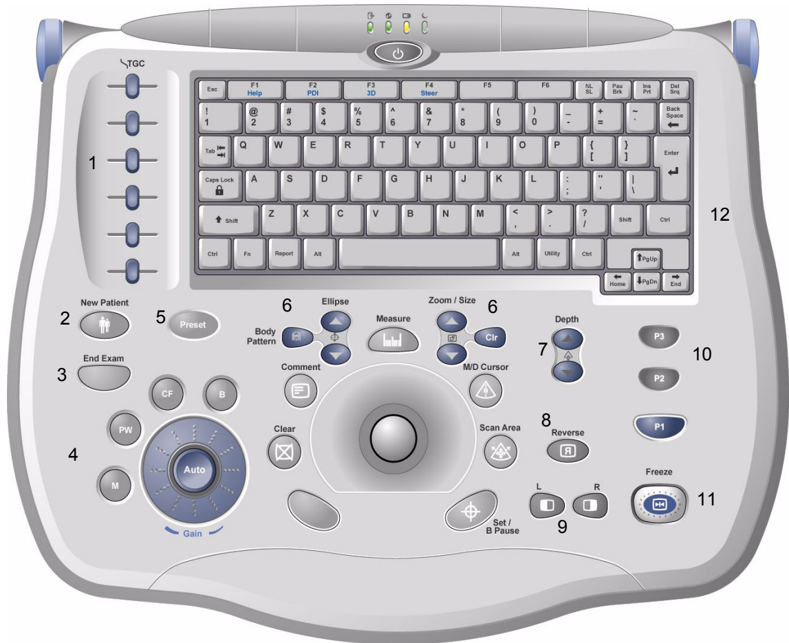
Figure 4-47 Control Panel Tour
