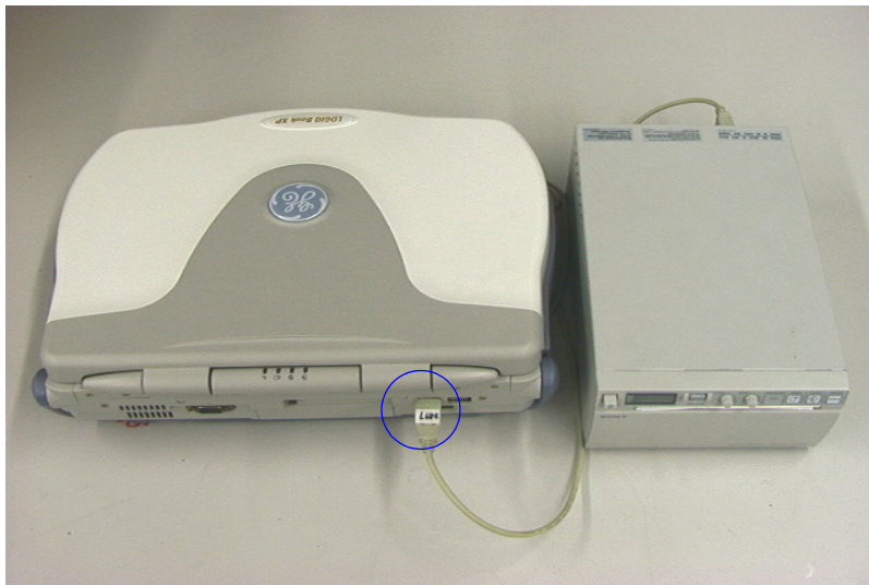
Figure 3-13 Connect B/W printer to the system
