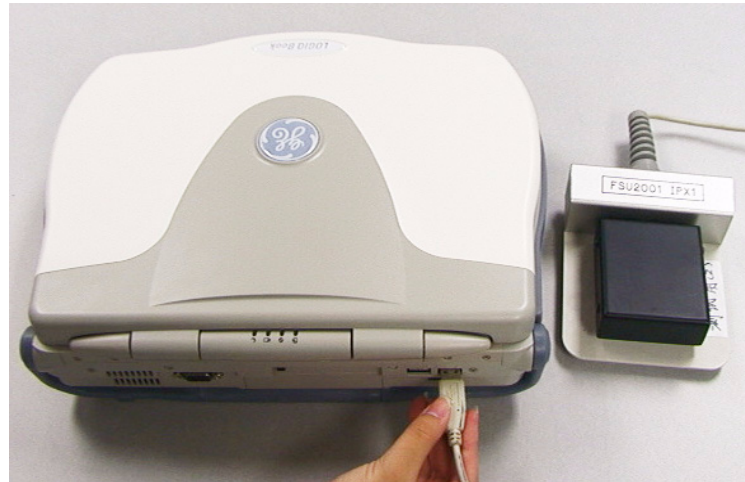
Figure 3-16 Connect Footswitch to the system
