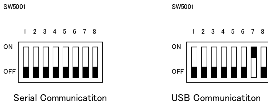
Figure 6-51 MD-3000 Dip Switch
