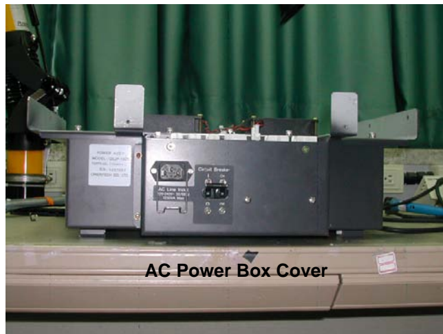
Figure 8-182 Unscrew 6 screws to remove AC Power Box
