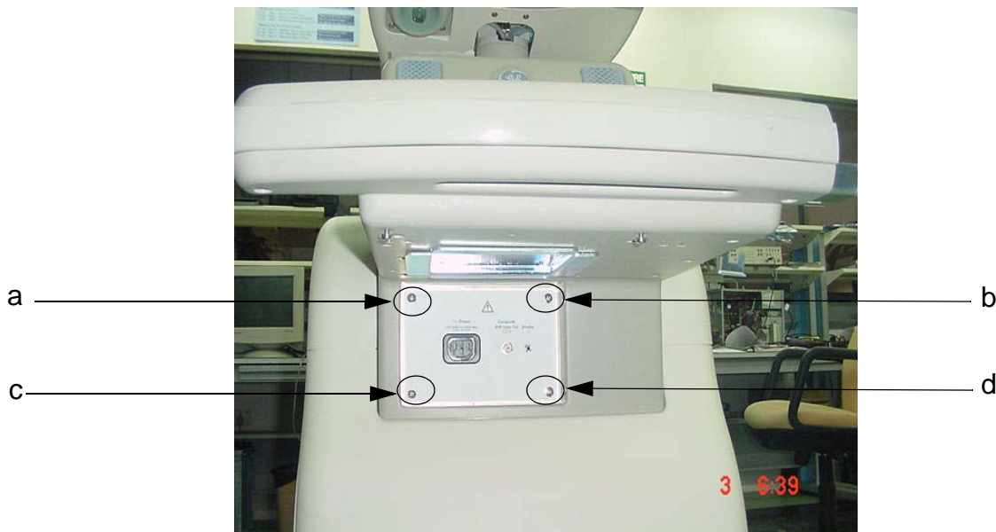
Figure 8-47 Front Panel Disassembly
