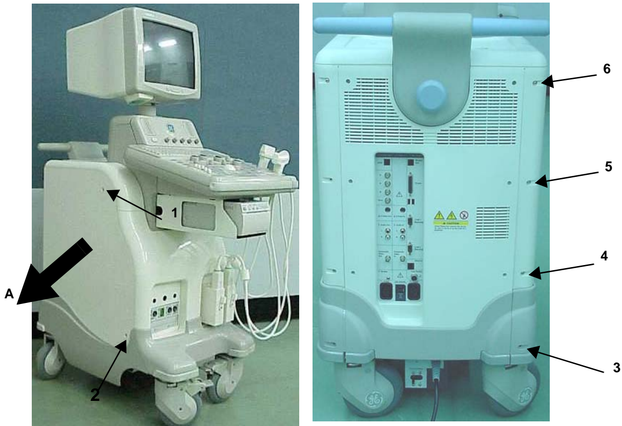
A. After removing the screws(1-6), then remove the left cover in the direction of arrow.
