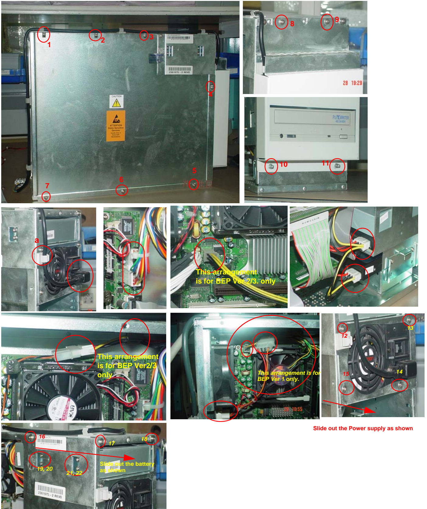
Figure 8-57 BEP Power Supply Replacement
